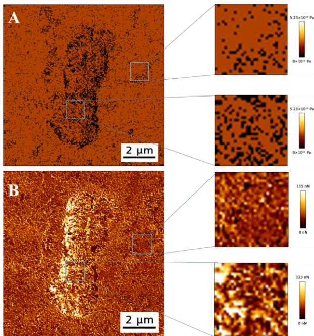
Fig.3. The adhesion image (A) and Young's modulus image (B) of dried chromosome.
