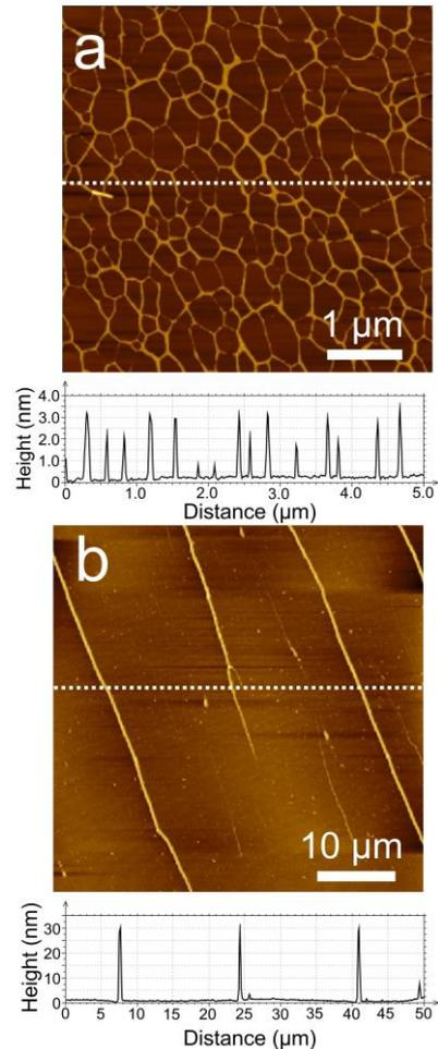
**Figure 2** The AFM morphological images of DNA molecules deposited on (a) bare mica and (b) Au layer surfaces. Below the morphological images are their corresponding height profiles. The DNA molecules were stretched on the Au layer surface.
