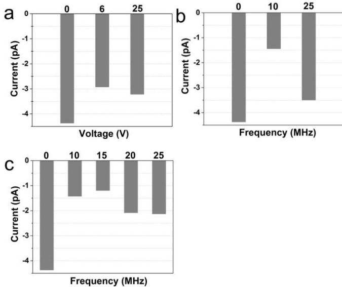
**Figure 5** (a) Current distributions of DNA strands under the effect of SMF with different intensities (0 V, 6 V and 25 V). (b) Current distributions of DNA strands under the effect of 5 V HFEF with different frequencies (0, 10 and 25 MHz). (c) Current distributions of DNA strands under the effect of 10 V HFEF with different frequencies (0, 10, 15, 20 and 25 MHz).
