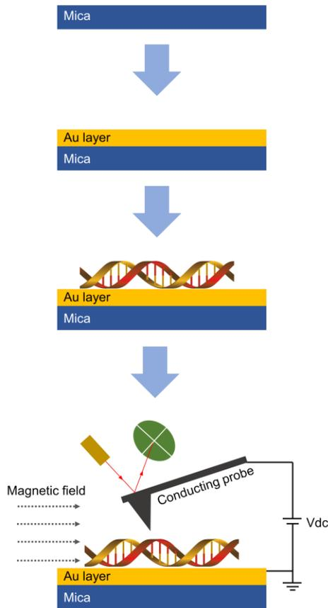
**Figure 1** The schematic diagram of DNA conductivity under the effects of magnetic fields measured by C-AFM.
