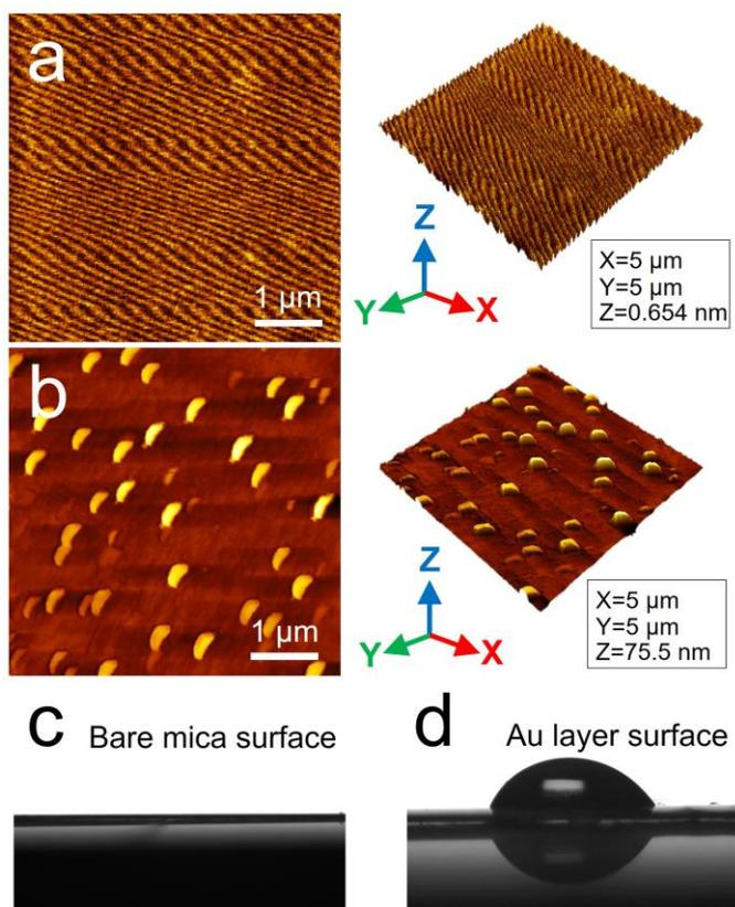
**Figure 3** The AFM images, 3D topographic maps of (a) bare mica and (b) Au layer surfaces. Pictures c and d are the water droplet on the bare mica surface and Au layer surface, respectively.
