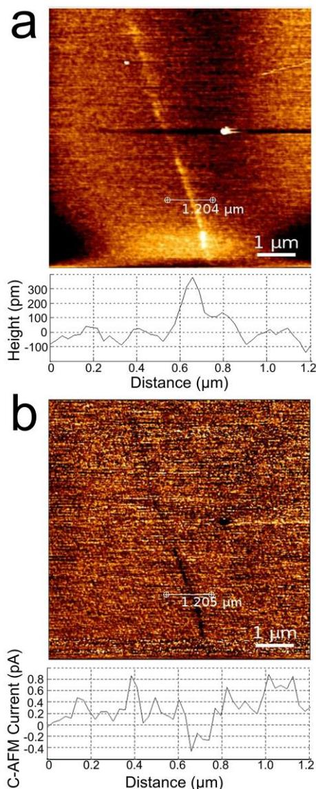
**Figure 4** The morphological (a) and current (b) images of DNA strand on the Au layer surface tested by C-AFM without the effect of magnetic field. The line charts are the corresponding height and current profiles, respectively.
