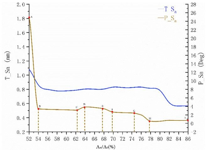
**Fig. 5.** Influence of the change of  $A_{st}/A_0$  percentage value on PR-AFM imaging. The blue line is the curve of the roughness  $T_{S_a}$  of the topography with the change of the percentage of  $A_{st}/A_0$ . The dark yellow line is the curve of the roughness  $P_{S_a}$  of the phase image with the change of the percentage of  $A_{st}/A_0$ .
