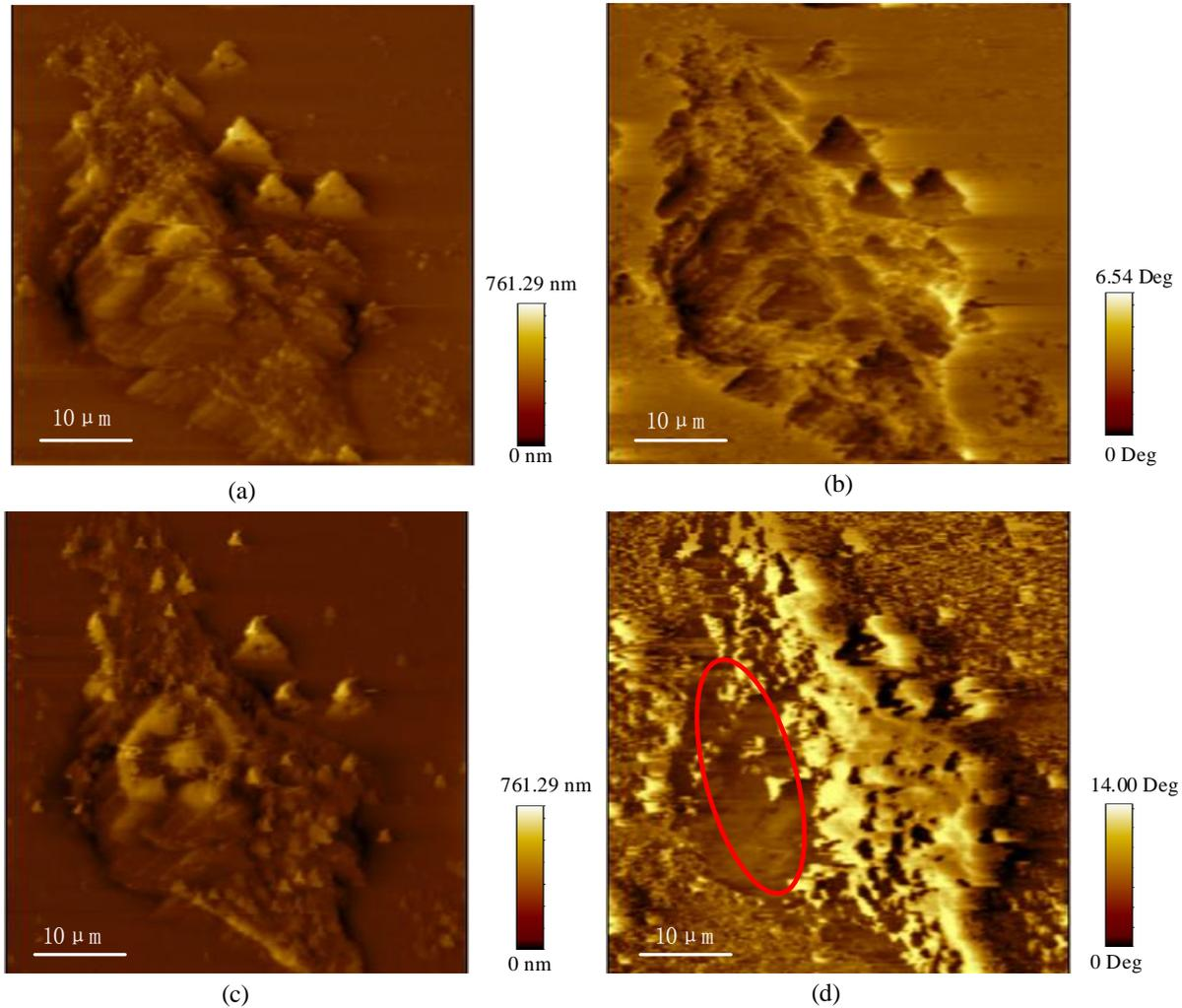
**Fig. 6.** PR-AFM scanning images of SMC7721 cells with different  $A_{st}/A_0$  percentage values. (a) and (b) are the topography and phase images of SMC7721 cells with the  $A_{st}/A_0$  percentage value of 72%. (c) and (d) are the topography and phase images of SMC7721 cells with the  $A_{st}/A_0$  percentage value of 54%. The structure at the bottom of the cell can be seen in the left red area of the phase image (d).
