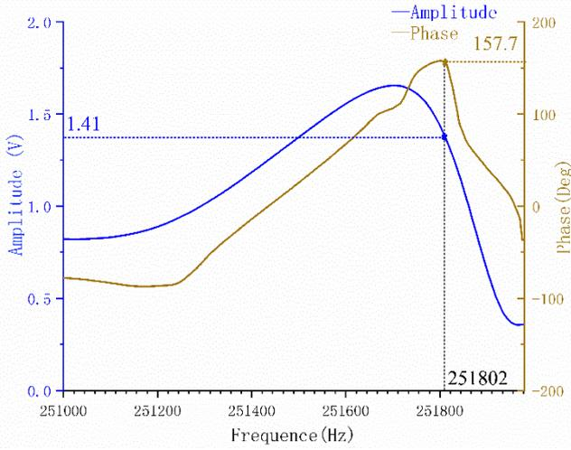
**Fig. 2.** Phase spectrum and amplitude spectrum of TM-AFM probe working near the phase resonance peak. The frequency at the phase resonance peak of the probe is 251802 Hz, the phase value is 157.7°, and the amplitude is 1.41 V.
