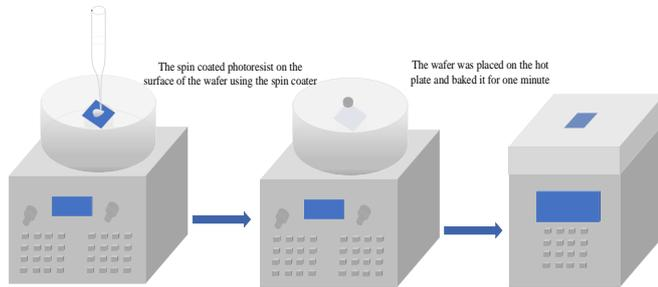
**Fig. 3.** Spin-coated photoresist sample preparation process. the spin coated photoresist SU-8-2000.5 on the surface of the wafer using the spin coater. After the coating, the wafer was placed on the 95° hot plate and baked it for one minute.
