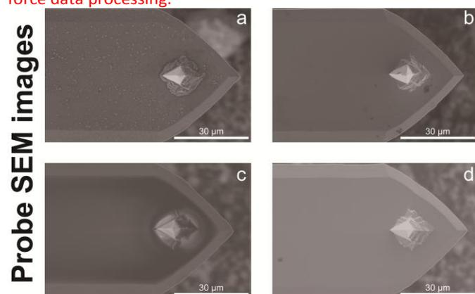
**Fig. 1** SEM images of the AFM probe cantilever contamination after being immersed in different liquids for 3 h. SEM was working at the high vacuum mode (5000 $\times$  magnification, spot: 3.0, HV: 3.00 kv, chamber pressure: 6.72 e-4 Pa).
