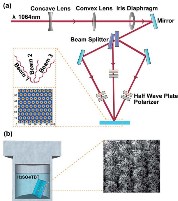
Fig. 1 (a) Schematics of experimental setup for the laser interference ablation. The primary laser beam was split into three coherent beams (beams 1, 2 and 3). The inset is the simulated laser intensity distribution of the laser interference ablation. (b) Schematic illustration of the hydrothermal reaction.
