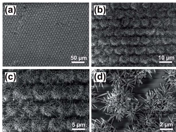
Fig. 3 SEM images of the 2D TiO<sub>2</sub> clusters with different magnifications.
