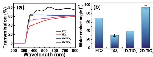
Fig. 4 (a) Transmissions of the bare FTO substrate, unpatterned TiO<sub>2</sub> nanowire arrays, (b) contact angles of the bare FTO substrate, unpatterned TiO<sub>2</sub> nanowire arrays, 1D and 2D TiO<sub>2</sub> clusters.
