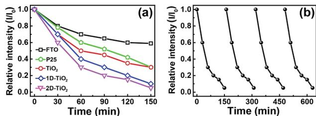
Fig. 5 (a) Photocatalytic decomposition of rhodamine B on the bare FTO substrate, P25 TiO<sub>2</sub> film, unpatterned TiO<sub>2</sub> nanowire arrays, 1D and 2D TiO<sub>2</sub> clusters. (b) Recyclability test of degradation curves of 2D TiO<sub>2</sub> clusters.
