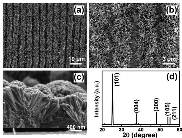
Fig. 2 (a) and (b) Top-view and (c) cross-sectional SEM images of 1D  $\text{TiO}_2$  clusters. (d) XRD pattern of 1D  $\text{TiO}_2$  clusters on the FTO substrate.
